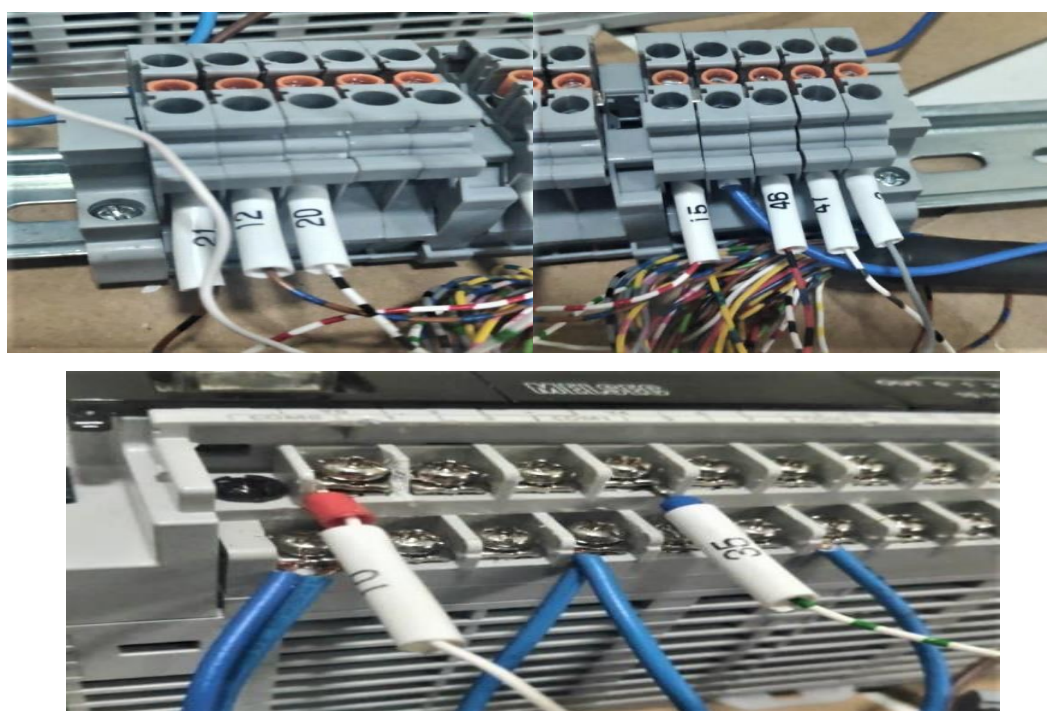
Figure 5.6: (From Left) Figure a: +24 V connection; Figure b: 0 V connection; Figure c: Pulse/Sign Pins.
